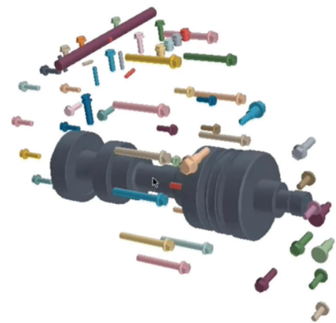
Figure 7. The ML algorithm automatically identifies and tags the nuts and bolts for deletion, even if it has not seen this geometry before.
